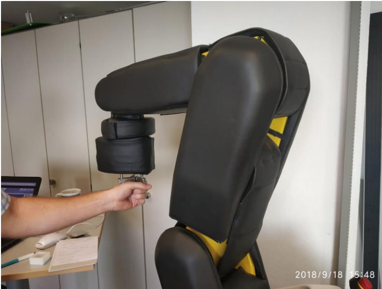
APAS Collaborated Industry Robot (No casing required, Touch sensitive)
