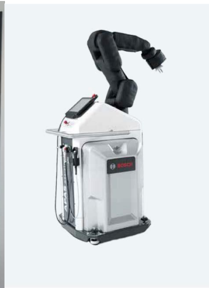
APAS Collaborated Industry Robot (No casing required, Touch sensitive)
